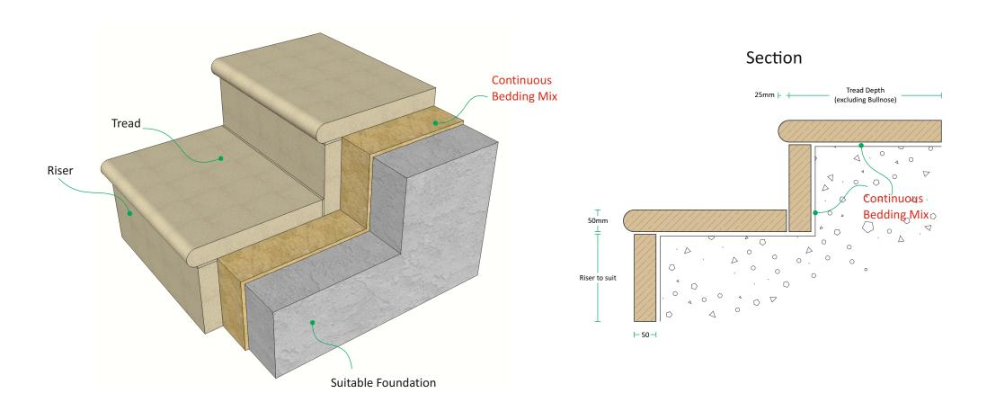
Our bullnose treads are supplied in 1000mm and 500mm lengths for cutting to final lengths on site with depths to suit all applications up to 550mm excluding the 25mm bullnose. Risers are supplied in 500mm lengths with various heights up to 200mm. Our steps are suitable for light domestic use and should be installed on a continuous mortar bed.
