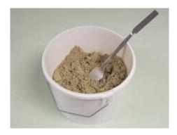
Step 3. The mix is ready when it reaches the consistency of damp sand. It will also just hold itself together when squeezed into a ball.
