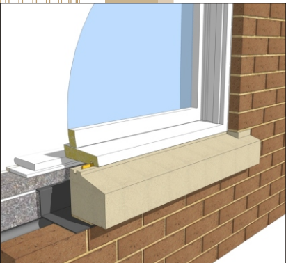
Typical installation detail
