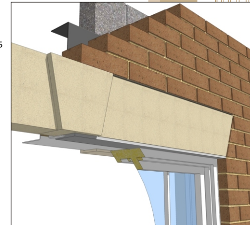
Typical installation detail
