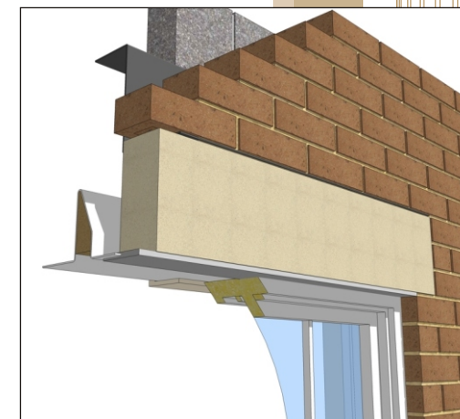
Typical installation detail
