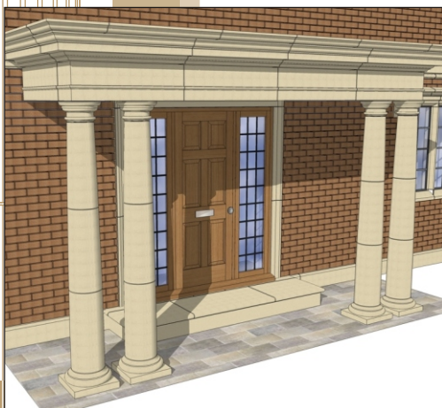
Typical installation detail
