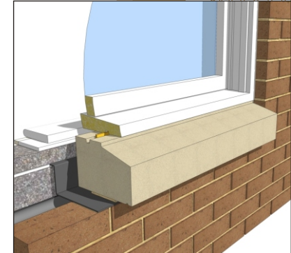
Typical installation detail
