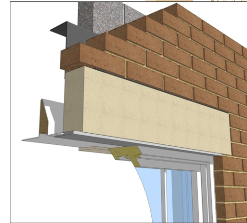
Typical installation detail
